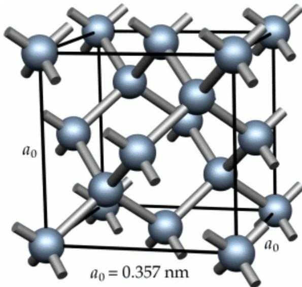
(FCC with additional atoms at  $(1/4, 1/4, 1/4)$ ,  $(3/4, 3/4, 1/4)$ ,  $(3/4, 1/4, 3/4)$ ,  $(1/4, 3/4, 3/4)$ ; this is a very important crystal structure in science and engineering because silicon takes on this structure)
